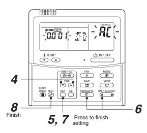
**4** Push the TIME **●** / **●** buttons repeatedly to change the value of the indoor unit address in SET DATA.
