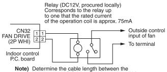
indoor control P.C. board and the relay within 2m.
