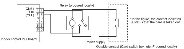
Note) Determine the cable length between the indoor control P.C. board and the relay within 2m.
