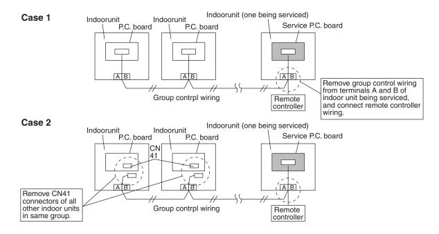
\* Be sure to restore the temporarily removed group control wiring and CN41 connectors to their initial states after Procedure 3 has been completed.
