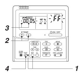
Clearing an error of the indoor unit Push the button on the remote controller. (Only the error of the indoor unit controlled by the remote controller will be cleared.)
