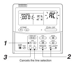
If no number appears on UNIT No., no outdoor unit exists on the line. Push button and select another line following step 2.
