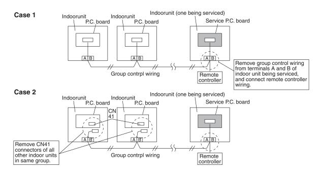
\* Be sure to restore the temporarily removed group control wiring and CN41 connectors to their initial states after Procedure 3 has been completed.
