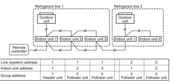
In the example above, disconnect the remote controller connections between the indoor units and connect a wired remote controller to the target unit directly before address setting.
