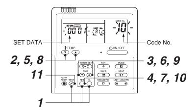
Pair the indoor unit to set and the remote controller one-to-one.
