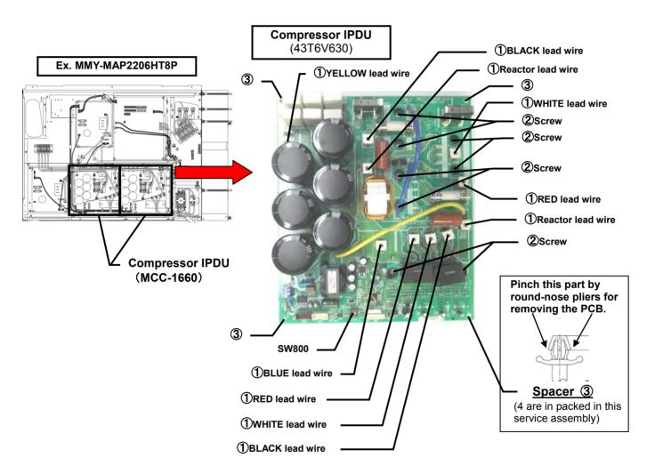
(5) Set the DIP switch (SW800) setting of the service board to match the switch setting from the original PCB.
