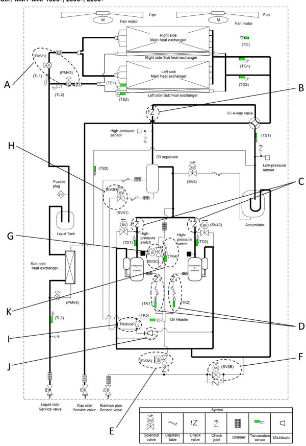
%) C/O models don't have 4-way valve and coil. However, MMY-MAP\*\*06T8(J)P-E models don't have only 4-way coil.
