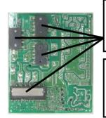
Uniformly apply the Silicone Thermal Grease to the heat dissipating surfaces of the IPM (Q201) and rectifier (DB01, DB02, DB03).
