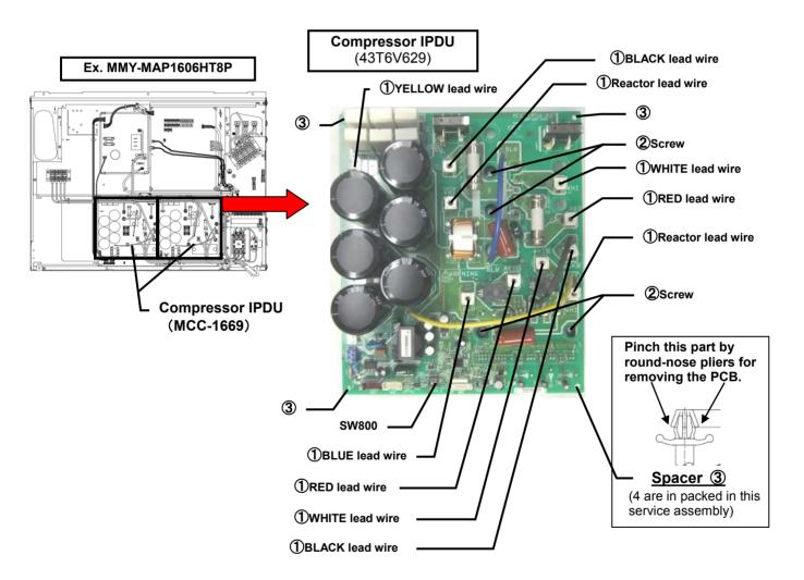
(5) Set the DIP switch (SW800) setting of the service board to match the switch setting from the original PCB.
