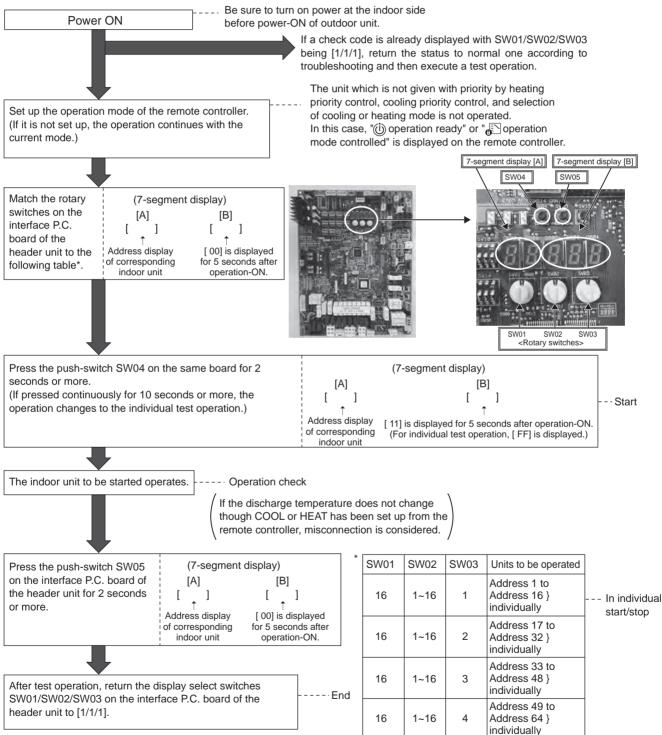
**NOTE)** The individual test operation returns to the normal operation after 60 minutes.
