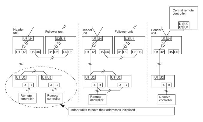
2 Turn on the indoor and outdoor units of the refrigerant line for which you want to initialize the addresses. About one minute after turning on the power, confirm that the 7-segment display on the header outdoor unit indicates "U.1. - - -" and operate the interface P.C. board on the header outdoor unit of the refrigerant line as follows.
