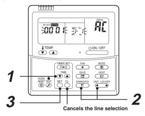
If no number appears on UNIT No., no outdoor unit exists on the line. Push  $\overset{\alpha}{\bigcirc}$  button and select another line following step **2**.
