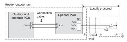
SW1: Cooling mode specified input switch SW2: Heating mode specified input switch
