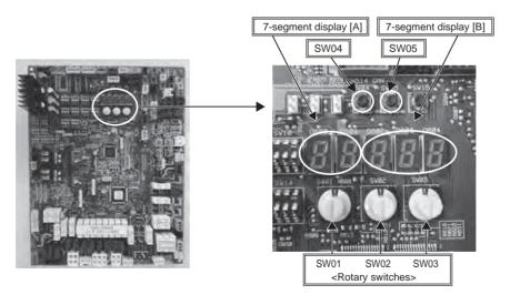
(5) Individual start/stop (ON/OFF) individual test operation function
