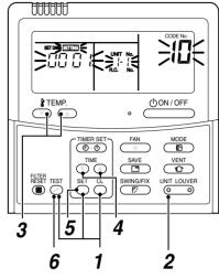
2 Each time the button is pushed, one of the indoor unit Nos. under group control is displayed in turn. Select the indoor unit whose setting is to be changed.
