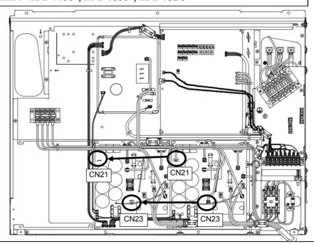
Change the connection of wiring which is connected to the CN21, 23 of Comp-IPDU2
