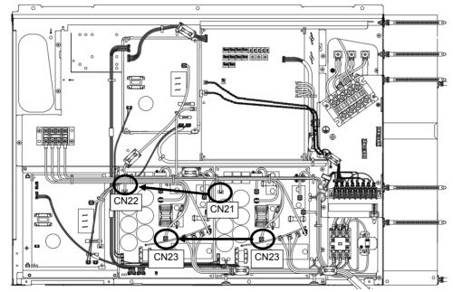
Change the connection of wiring which is connected to the CN21, 23 of Comp-IPDU2
