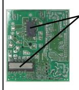
Uniformly apply the Silicone Thermal Grease to the heat dissipating surfaces of the IPM (Q201) and rectifier (DB01).
