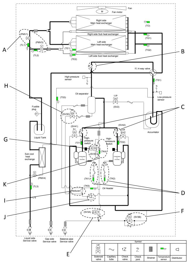
※) C/O models don't have 4-way valve and coil. However, MMY-MAP\*\*06T8(J)P-E models don't have only 4-way coil.
