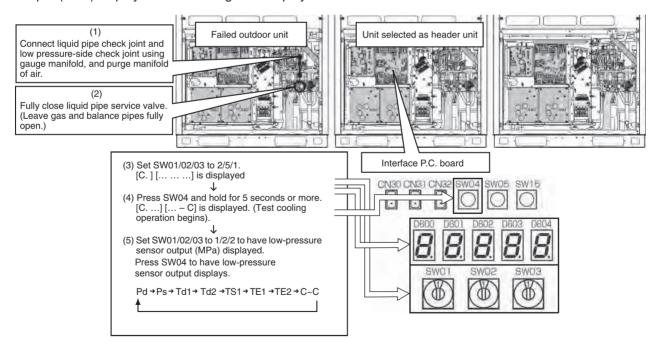
(6) Approx. 10 minutes after the system starts up, fully close the gas pipe service valve of the failed outdoor unit. [Selection of outdoor unit for pressure adjustment]
