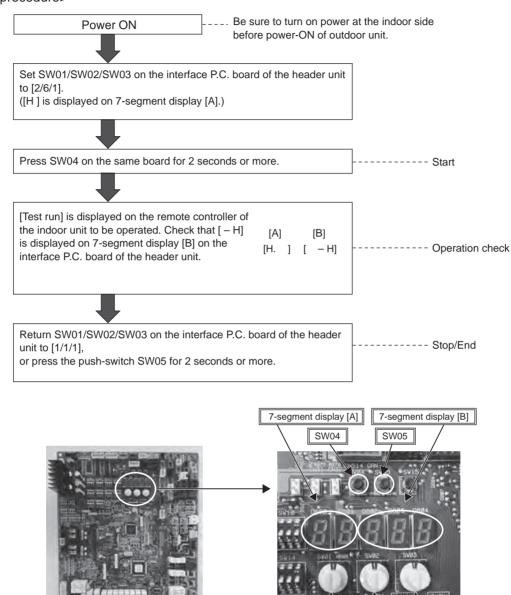
**NOTE)** The test operation returns to the normal operation after 60 minutes.
