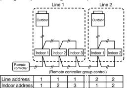
In the above example, where remote controllers are not yet wired, set the address manually after individually connecting the wired remote controller.
