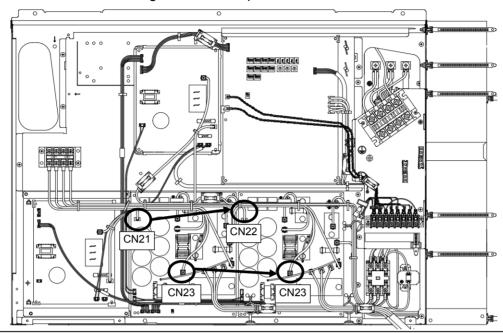
Change the connection of wiring which is connected to the CN21, 23 of Comp-IPDU1
