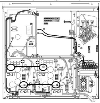
Change the connection of wiring which is connected to the CN21, 23 of Comp-IPDU2
