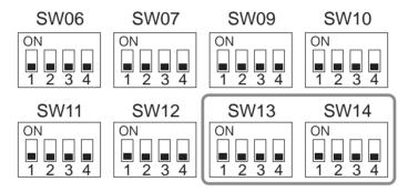
Line address switches on the outdoor interface PC board (O: switch on, X: switch off)
