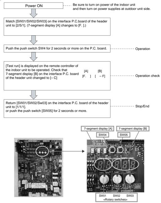
**NOTE)** The test operation ends after 60 minutes and the operation returns to normal status.
