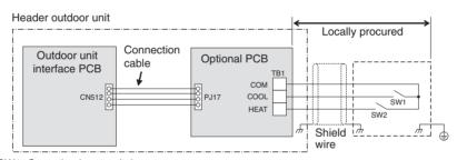
SW1: Operation input switch SW2: Stop input switch
