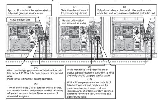
This is the end of the refrigerant recovery operation. Set SW01/02/03 of the header unit back to 1/1/1.
