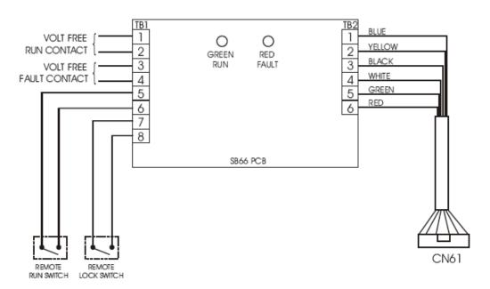
Jumper J01 must be removed from the indoor PCB to enable switching operation.
