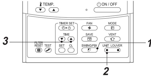
**1 Push** **for at least four seconds when the air conditioner is not working.**
