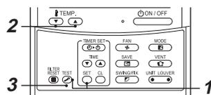
**1** When **SET** and **TEST** buttons are pushed at the same time for 4 seconds or more, the following display appears.
