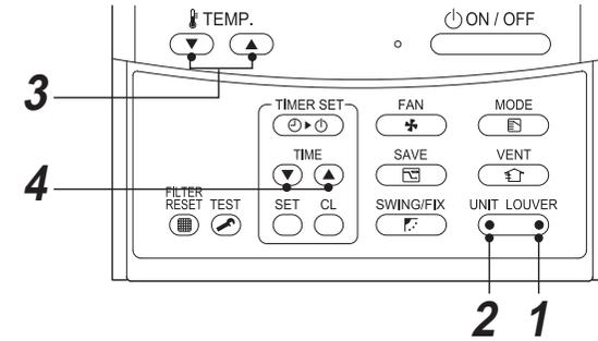
**1 Push** **(right side of the button) for at least four seconds when the air conditioner is not working.**
