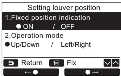
**1** Push the [ ] / [ ] button to select “5. Setting louver position”, then push the “ Set” [F2 F2] button.
