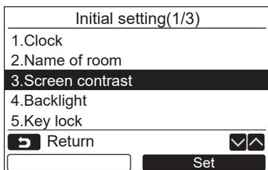
**1** Push the [ ^ ^ ] / [ v v ] button to select “3. Screen contrast” on the “Initial setting” screen, then push the “Set Set” [F2] button.
