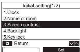
**1** Push the [ ^ / ^ ] / [ v / v ] button to select “3. Screen contrast” on the “Initial setting” screen, then push the “ Set” [■ F2] button.
