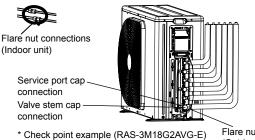
Check point example (RAS-3M18G2AVG-E) Flare nut connections (Outdoor unit)
