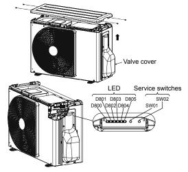
3. Turn on the circuit breaker to supply electricity. In the initial LED display status, D805 is lighted as below.
