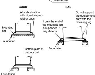
Support the bottom surface of the mounting leg that is in contact with and underneath the bottom plate of the outdoor unit.
