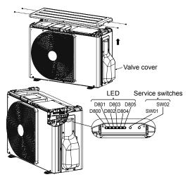
3. Turn on the circuit breaker to supply electricity. In the initial LED display status, D805 is lighted as below.
