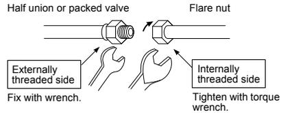
**2** As shown in the figure, be sure to use two wrenches to loosen or tighten the flare nut of the valve on the gas side. If you use a single crescent, the flare nut cannot be tightened to the required tightening torque.
