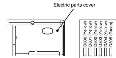
Inspection window through which to check the LED displays
