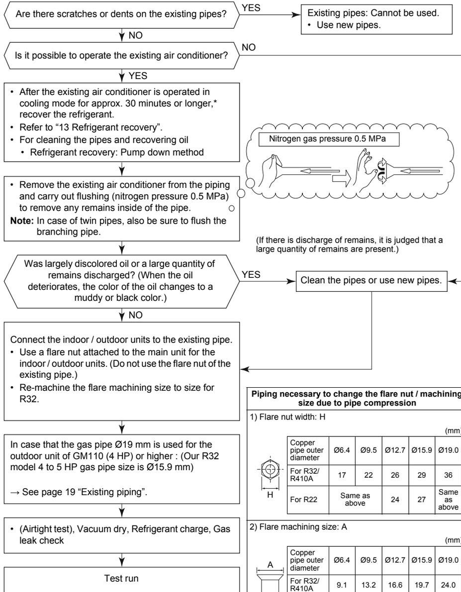
**Piping necessary to change the flare nut / machining size due to pipe compression**
