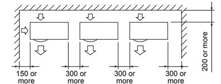
The height of the obstacle should be lower than the height of the outdoor unit.
