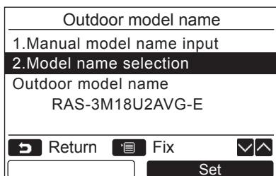
**1 Push the [ ]/[ ] button to select “2. Model name selection” on the “Outdoor model name” screen, then push the “ ” Set [ ] F2] button.**
