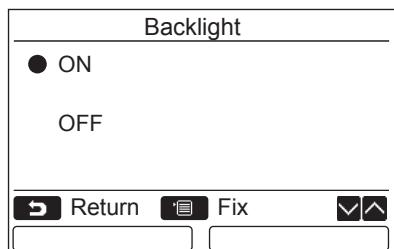
**1** Push the [ $\wedge \wedge$ ] / [ $\vee \vee$ ] button to select “4. Backlight” on the “Initial setting” screen, then push the “**Set**” [F2] button.
