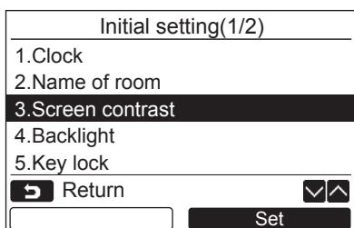
**1** Push the [ ]/[ ] button to select “3. Screen contrast” on the “Initial setting” screen, then push the “Set” [F2] button.
